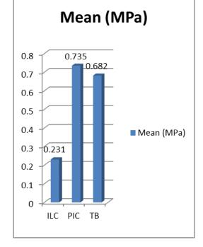
Table II Mean tensile strength of cement in group II
